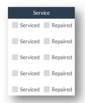
SERVICED is any maintenance activity on a device that DOES NOT TRIGGER A NEW CALIBRATION. This includes but is not limited to LED screens, nozzles, hoses and a routine calibration test (aka: performance test/device inspection).
